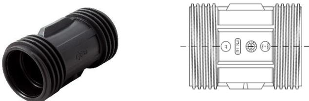
Printed in PP copolymer type B, UV-resistant thanks to the special black pigmentation. Strong design, it is provided with a large range of products (tee, couplings, elbows, etc.) designed to meet the different needs of the installer. The threaded bodies provide, starting from r.1 1/4 ", a metal reinforcement on the external part of the thread made of steel AISI 430: this is to make it stronger and secure the threaded joint.
