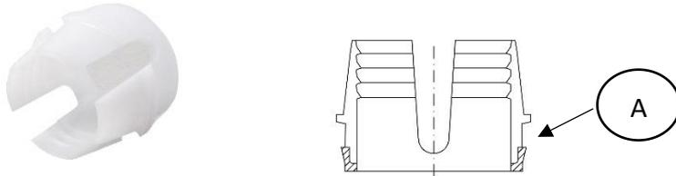
Printed in POM (polyoxymethylene) white. The raw material is particularly rigid and therefore suitable for the grafting on the pipe in PE. **The special "flower" shape of the ring allows 4 grip points on four rows of teeth, a seal ring and therefore safer and integral with the pipe. The ring is also provided with a tooth (A) retaining the body: this allows the connection to the body at the moment of the removal of the ring, avoiding unpleasant "fall" of the ring.**
