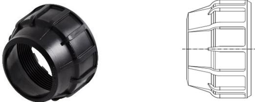
Even in large diameters the rings are strong and the ribs are even more marked to facilitate the use of the key for tightening. Moulded in PP copolymer type B, UV-resistant thanks to the black pigmentation.
