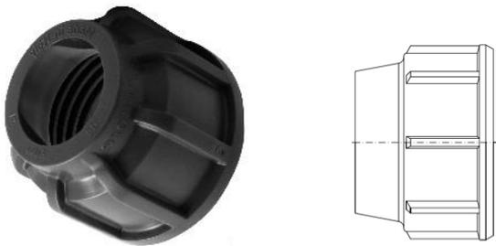
The compression fitting ASTORE has a highly ergonomic design, it has ribs that facilitate the grip for both hands and for any key for tightening. It is printed in PP copolymer type B and thanks to the special black pigmentation is UV-resistant.
